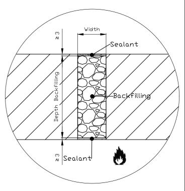
Soudafoam® FR HY backfilling at an offset of 3 mm and Firecryl® FR sealant at both sides.
