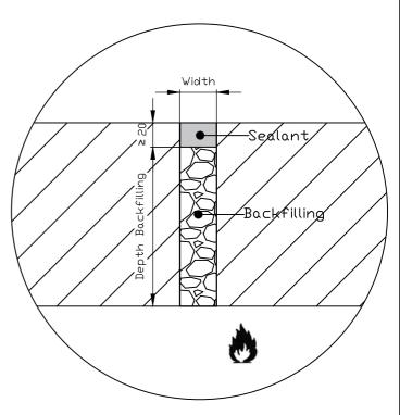
Soudafoam® FR HY backfilling flush with the exposed side and sealant at the unexposed side.
